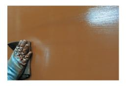
KIKUKAWA's original "FURUMI" finishing allows us to create the look of aged metal right from the beginning. A mixture of sulfurizing and surface-roughening processes are employed to create a sense of profoundness and feeling of luxury. This finish is particularly favored for European designs.
